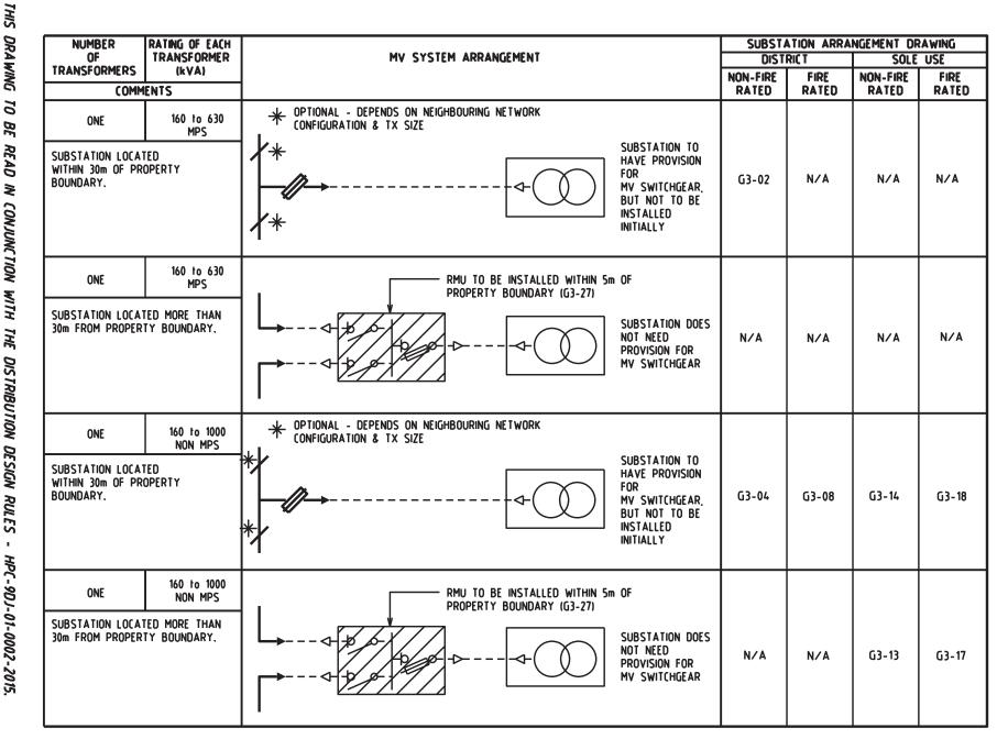
DISTRIBUTION CONSTRUCTION STANDARDS 11kV OVERHEAD SUPPLY DISTRICT AND SOLE USE SUBSATION, TYPICAL URBAN
